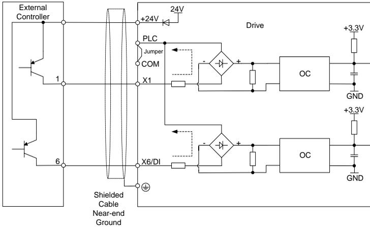
Fig. 3-18 Internal power supply open collector PNP connection
