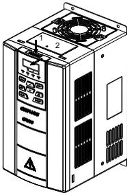
Fig. 3-3 Remove the control panel
