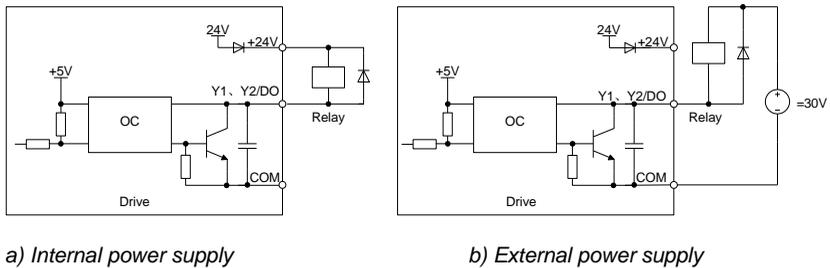
Fig. 3-21 Wiring when Y1 and Y2/DO drive relay
