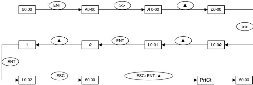
Fig. 4-15 Flow chart of locking control panel
