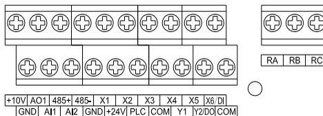
Fig. 3-13 Lay-out of control terminals
