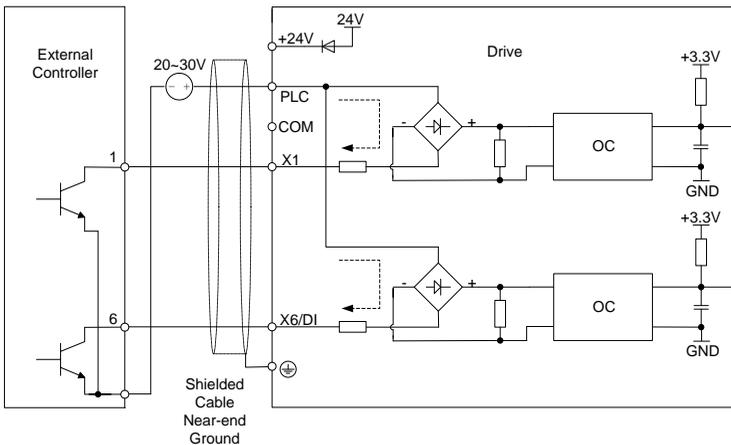
Fig. 3-17 External power supply open collector NPN connection
