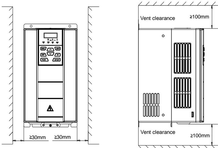
Fig. 3-1 Minimum mounting clearances of 600-2T7.5B and below, 600-4T15G/18.5LB and below
