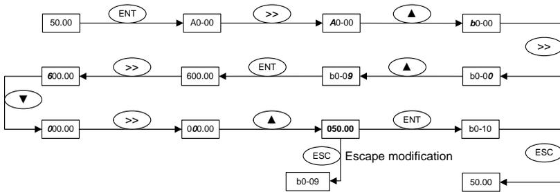
Fig. 4-12 Flow chart of upper limit frequency modification
