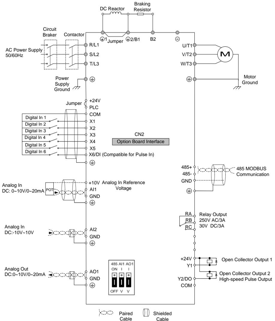
Fig. 3-12 Wiring diagram
