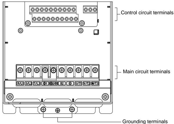
Fig. 3-10 Terminal configuration
