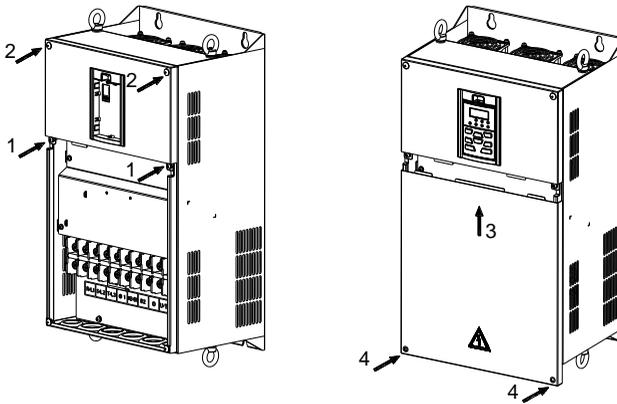
*Fig. 3-8 Mount the upper and lower covers*
