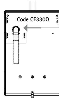
For rear installations, both with the FRONTAL air expulsion (fig. E) and with the UP air expulsion (Fig. F), must be used the rear installation kit for wall-mounted QB in thermoplastic material Cod. CF330Q
