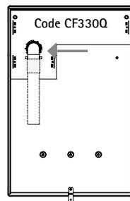
**F. REAR:** REAR dust inlet and air Expulsion DUCTED upwards
