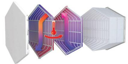
The DVUE units are equipped with a counter-flow enthalpy heat exchanger. In the cold season the extract air heat and moisture are transferred to the supply air stream through the enthalpy membrane. Heat recovery minimises heat losses from ventilation.
