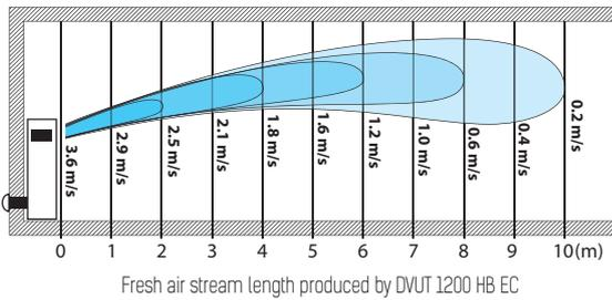
Fresh air stream length produced by DVUT 1200 HB EC
