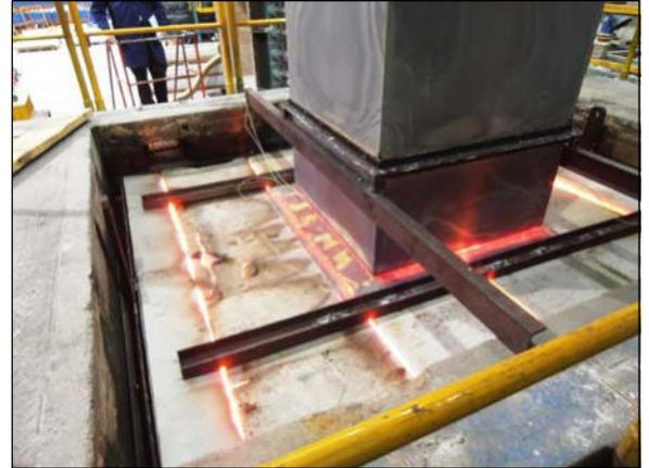
**Series 100 fire damper during a horizontal fire test**
