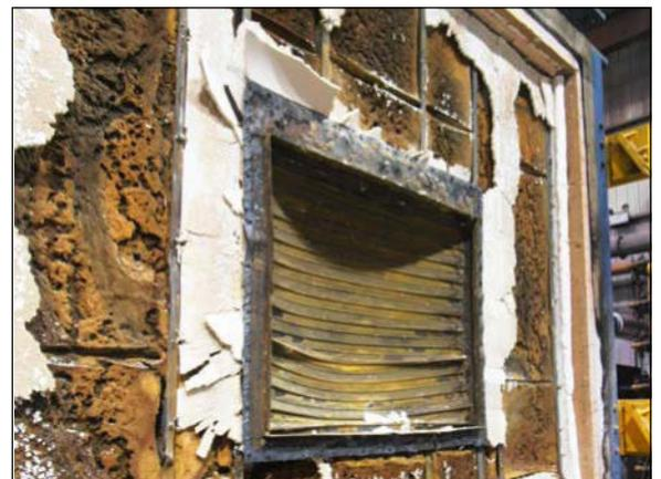
**Remains of a drywall partition after a fire test**
