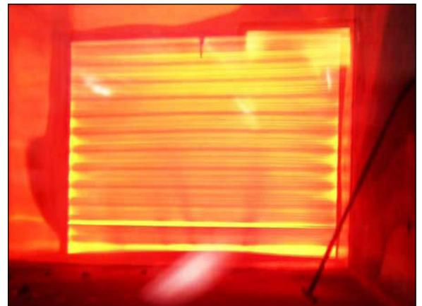
**Damper blades glowing during a vertical fire test**
