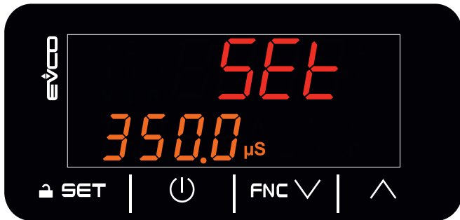
Fig. 4. First start-up - Setting the electrical conductivity
