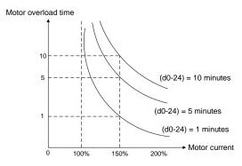
Fig. 6-39 Motor protection curve for ordinary motor running at 50Hz
