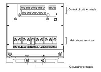
Fig. 3-10 Terminal configuration
