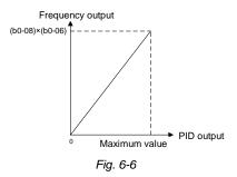
When b0-05 is set to 1 (relative to master frequency): When AI1, AI2, EAI, or X6/DI pulse input is selected for auxiliary frequency command source, the frequency that corresponds to maximum value of these sources should be: [master frequency × (b0-06)].
