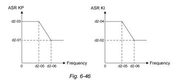
ASR parameters are normally adjusted in the following order: select appropriate switching frequency. Adjust proportional gain d2 -01 and integration time d2-02 at high speed, ensuring the system has no oscillation and meets the requirements of dynamic response characteristics. Adjust proportional gain d2-03 and integration time d2-04 at low speed, ensuring there is no oscillation at low speed and requirements of dynamic response characteristics are met.
