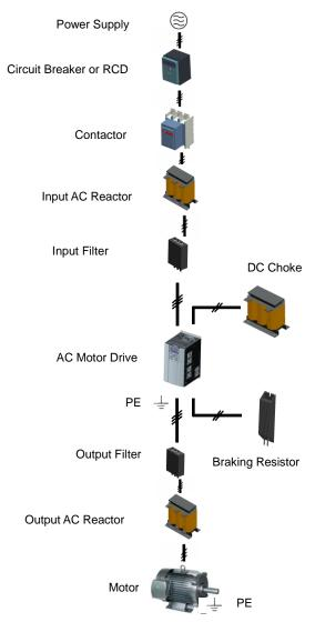
Fig. 3-9 Standard configuration of peripheral devices
