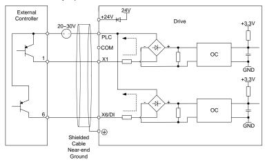
Fig. 3-19 External power supply open collector PNP connection
