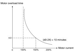
Fig. 6-40 Overload protection curve for ordinary motor running at 10Hz
