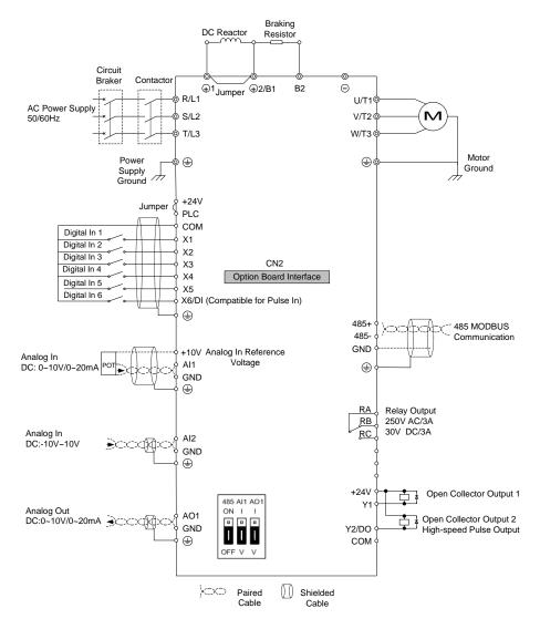
Fig. 3-12 Wiring diagram
