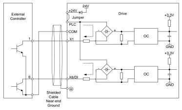
Fig. 3-16 Internal power supply open collector NPN connection
