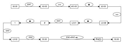
Fig. 4-15 Flow chart of locking control panel
