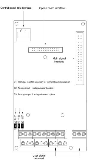
Fig. 3-11 Control board diagram
