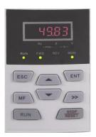
Fig. 4-6 Parameter value setting status (b0-02 is set to 49.83Hz)
