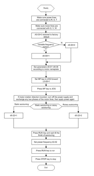
Fig. 4-17 Flow chart of first-time power up for asynchronous motor
