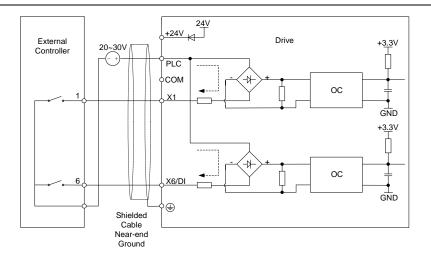
Fig. 3-15 External power supply dry contact
