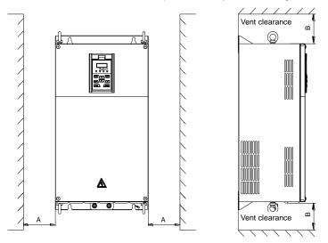
Fig. 3-2 Minimum mounting clearances of 600-2T11(B) and above, 600-4T18.5G/22L(B) and above
