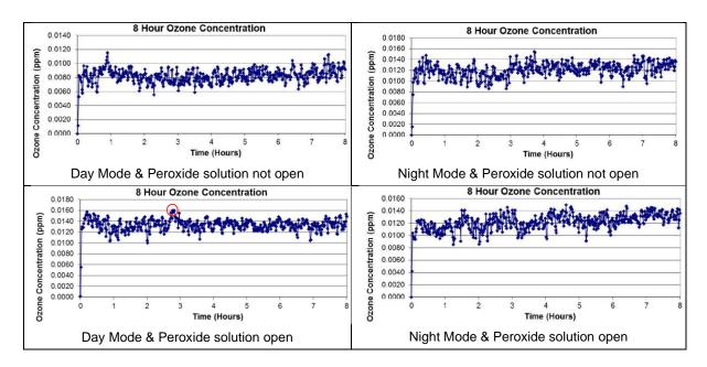
**Conclusions:** Wellisair has been found to meet the criteria with a maximum emission of 0,016ppm not exceeding the allowed concentration of 0.050ppm. Furthermore, a second Wellisair was not required to be tested according to UL867, as the first sample's maximum emissions were less than 0,030ppm, which satisfies the exception in the section 40.1.1.
