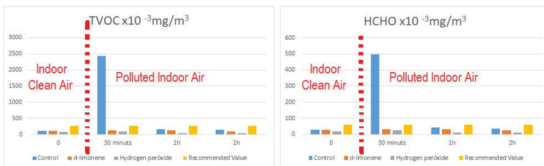
Figure 1. Air quality lectures before and after contaminating the room with the combustion of an incense stick, comparison of the safety and efficacy of Wellis in the elimination of VOCs and formaldehyde with hydrogen peroxide and limonene.
