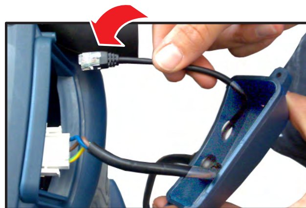
3 Insert the new wireless cable and connect it to the dedicated LM2 plug inlet.
