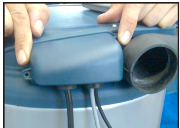
5 Insert the endless end into the cable gland where the wireless cable was already inserted.
