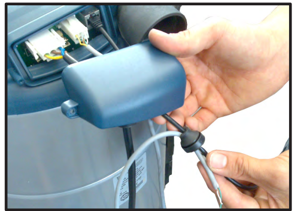
5 Insert the endless end into the cable gland where the wireless cable was already inserted.
