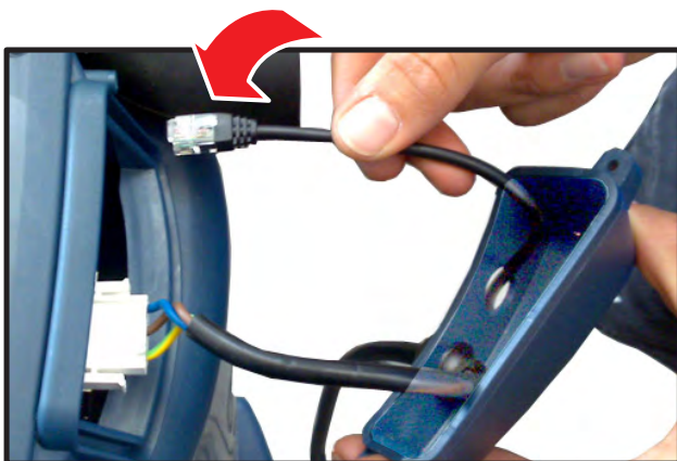
3 Insert the new wireless cable in the free hole and connect it to the dedicated LM2 plug inlet.
