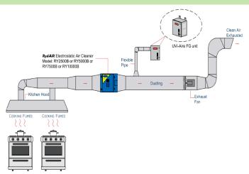
The FGA unit is a self contained unit with a 100mm diameter nozzle on one end to direct ozone to the required area by means of flexible or rigid ducts. Its small size makes it flexible for installation in various locations. As the FGA unit produces high levels of ozone, it operations should be interlocked with the exhaust fans for safety reasons.
