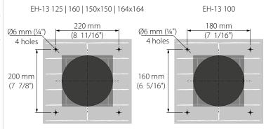
3. Insert the supplied expansion anchors 6 mm (1/4) x40 mm (19/16) into the holes.
