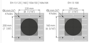
3. Insert the supplied expansion anchors 6 mm (1/4) x40 mm (19/16) into the holes.
