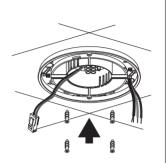
Connect the connectors and install the lamp on the fan casing by turning
