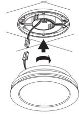
Connect the wires according to the Wiring diagram.
