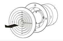
Mark the holes for fan fastening.
