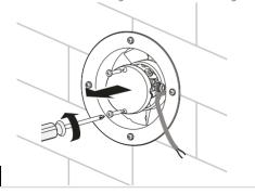
Fix the fan with the screws.
