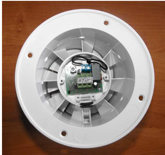
VENTS 100 PF2T turbo inside (PCB)
