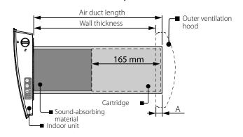
If the wall thickness is less than that in the layout of the blocks inside the wall, you can unfasten the fine filter holder and assemble the ventilator without it and without sound-absorbing material, as shown in the figure above.
