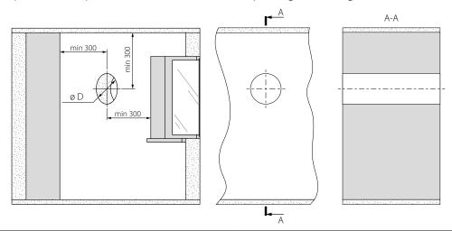
2. Insert the air duct in the wall. For ease of installation use the mounting wedges included in the delivery set.
