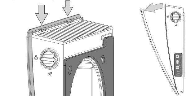
6. Remove the three retaining screws from the left cover to enable access to the terminals. Route the power wires through the appropriate cable glands.
