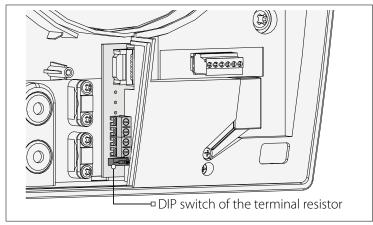
The DIP switch of the terminal resistor must be in ON position if the ventilator is the first or the last in the RS-485 network.
