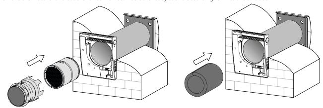
11. Install the front panel of the indoor unit.
