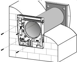
8. Route the power cable as figured below and connect the ventilator to power mains in compliance with the external wiring diagram, see section **Connection to power mains**. Secure the power cable with the clamp.
