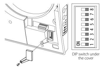
Prior to operating the ventilator set its operation modes using the DIP switch. It is located on the controller circuit board. To access the DIP switch, take off the front panel of the indoor unit and uplift the rubber plug that covers the switch.
