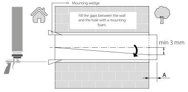
Install the air duct with the minimum slope of 3 mm downwards from the outer wall side.
